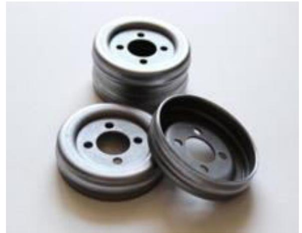
**Sleeves** are made from Aluminium blanks / Slugs & press drawn / extrude to form desired shapes & Sizes for various applications such as Suction, Discharge & Liquid Pipes. They are used for fixing End/connecting pipe of Auto air-conditioning Hoses & Pipes.
