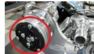
**Mozzo Hub** is press drawn part, made out of HRC sheet. It goes through multiple draw operations to form into the desired shape and size. It is supplied to Dayco and is used as a sub assembly part of Crankshaft Damper Pulley, which is installed on Automobile engines.
