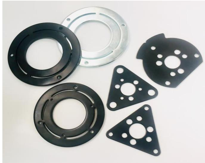
**Core Ring Assembly** is an important part of Auto Air-con Compressor. It is made of HRC & CRC sheets and drawn (single operation) into shape through a cut size blank. Core Ring Assy. is a part of Compressor clutch and it is fitted as a stationary electromagnetic coil, which is attached to the face of the compressor, behind the pulley.
